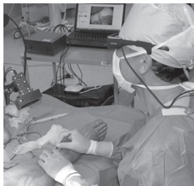
Fig.1. A surgeon is identifying ICG dyed lymphatic vessels through eye-glasses type display.
